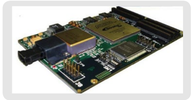
Custom Readout OptoRX mezzanine equipped with Altera FPGA
